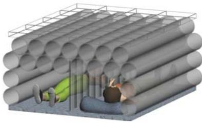
Fig. 5: Single/two-person deployable tube water radiation shielded sleep unit.
