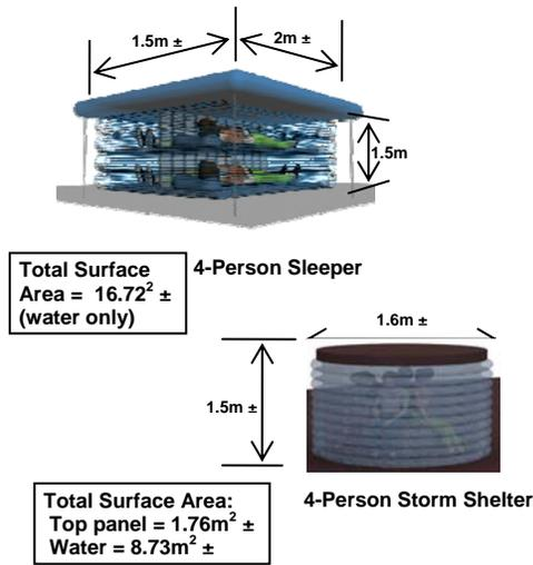
Fig. 16: Radiation shielding: hydraulic deployables.
