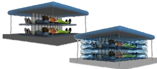
Fig. 4: Deployable drop-down sleeping units with water tube radiation shielding.
