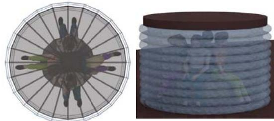
Fig. 8: Floor-deployed water tube radiation shelter.
