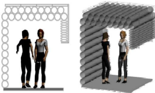
Fig. 7: Deployable walls with water tube radiation shielding.
