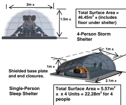
Fig. 17: Radiation shielding: erectable tents.
