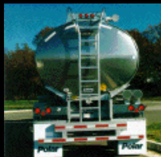
DOT-406 Elliptical Petroleum Trailer is a pressurized tank with an elliptical cross section.
