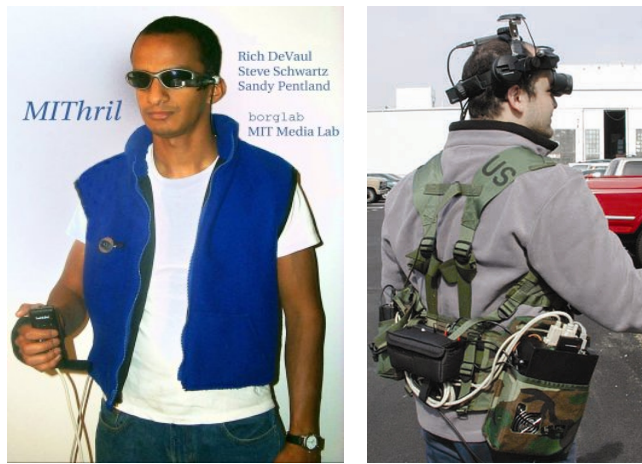
Figure 2: Examples of body-wearable technologies: MIT Media Lab's MITHril Project (left) and the Battlefield Augmented Reality System (right)
