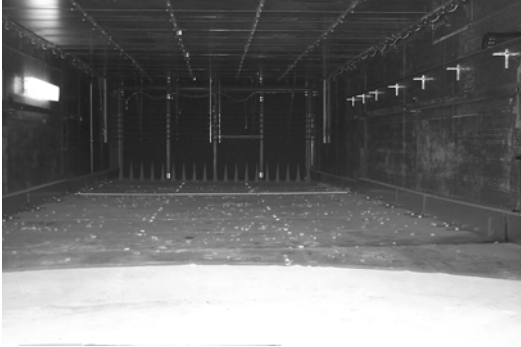
Figure 10. Interior of the wind tunnel at EPFL. Vortex generators and roughness elements produce a turbulent boundary layer.
