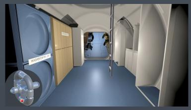
3) Crew ablutions module in the artificial gravity section, with washer/dryer unit, showers, basins and stowage
