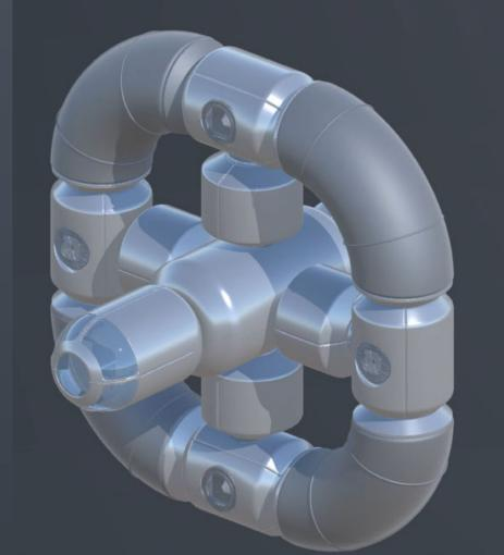
Aft isometric view of the Spaceship configuration, showing the Common Berthing Mechanisms and International Docking Adapters
