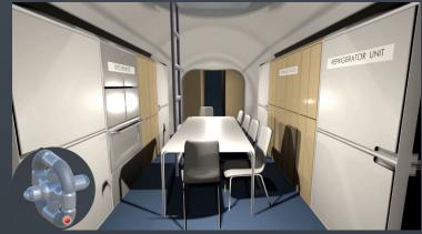
5) Crew galley module in the artificial gravity section, with a kitchenette for cooking various types of food, refrigeration units, stowage and foldable table and chairs
