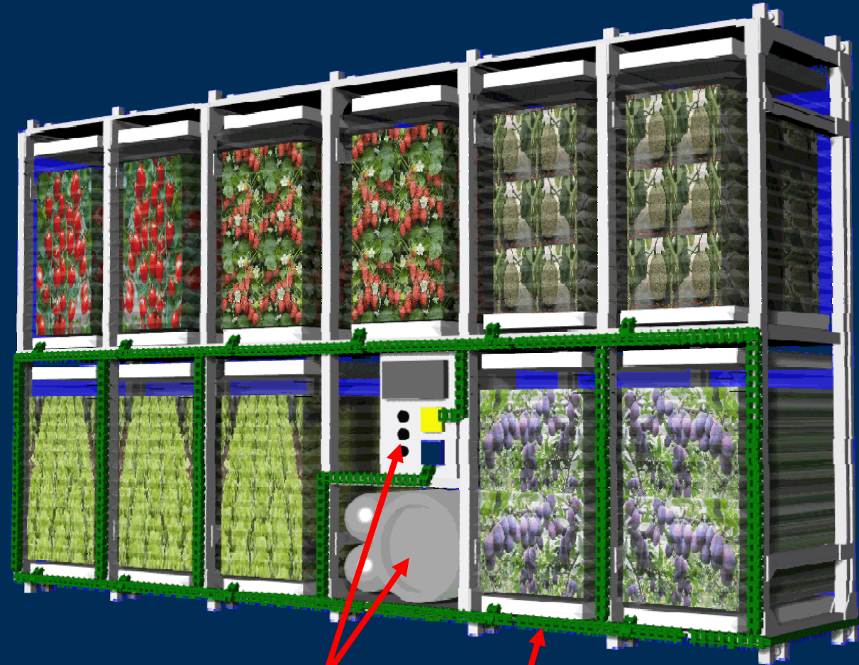
Fertilizer, CO2 tank, Control Assembly
