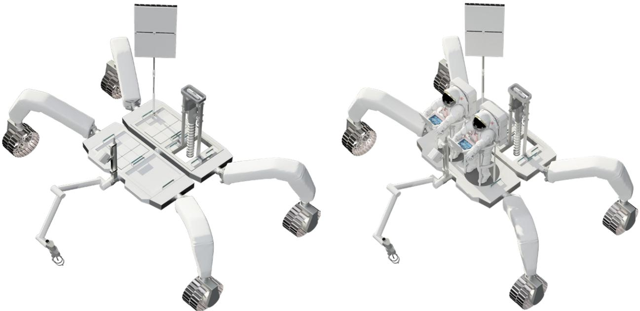
*Fig 1. The two main configurations: Teleoperated (Phase I) and Manned (Phase II)*
