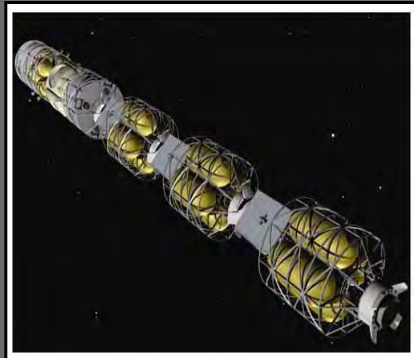
MLV Chemical Propulsion Stack
