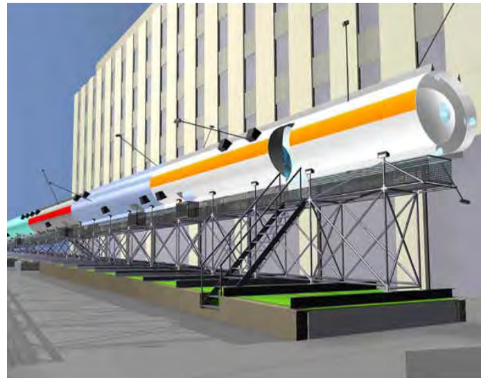
Tanks are Supported by a Steel Scaffold
