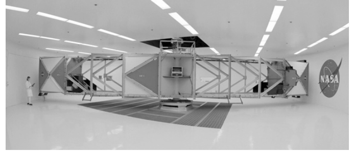
Fig. 3: The “20-G” centrifuge at Ames Research Center (courtesy of NASA).
