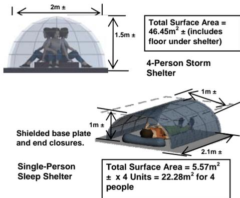
Fig. 17: Radiation shielding: erectable tents.
