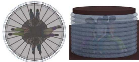
Fig. 8: Floor-deployed water tube radiation shelter.
