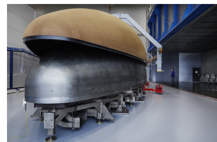
Figure 12. Payload Fairing Half Manufacture
