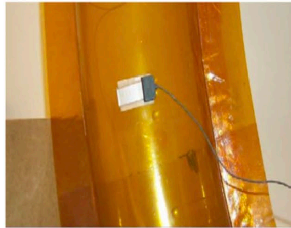
Figure 8: A shielded PVDF sensor bonded to the torus
