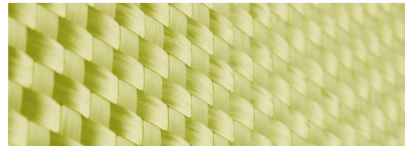
Close view of Kevlar strap at 90° cut
