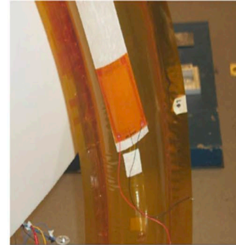
Figure 9: The MFC actuator attached to the torus
