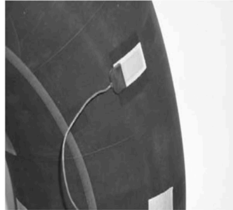
Figure 13: A shielded PVDF sensor bonded to the torus
